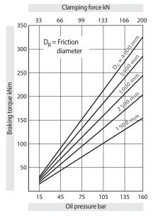
The braking torques shown in the diagram are based on a theoretical friction coefficient of 0,4.
