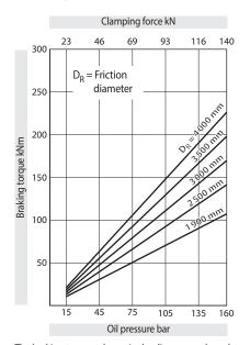
The braking torques shown in the diagram are based on a theoretical friction coefficient of 0,4.
