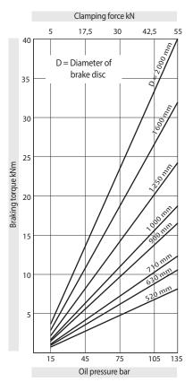
Oil pressure: Oil volume: Weight: min. 15 bar max. 125 bar max. 75 cm<sup>3</sup> ca. 60 kg
