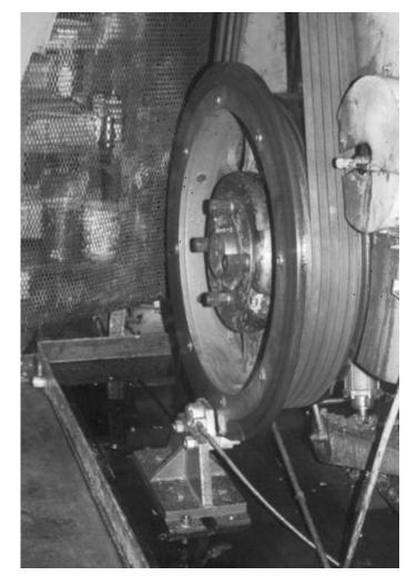
Direct drive application where the 225DP100 caliper is used to brake the flywheel of a 60 ton Header during the set-up process.
